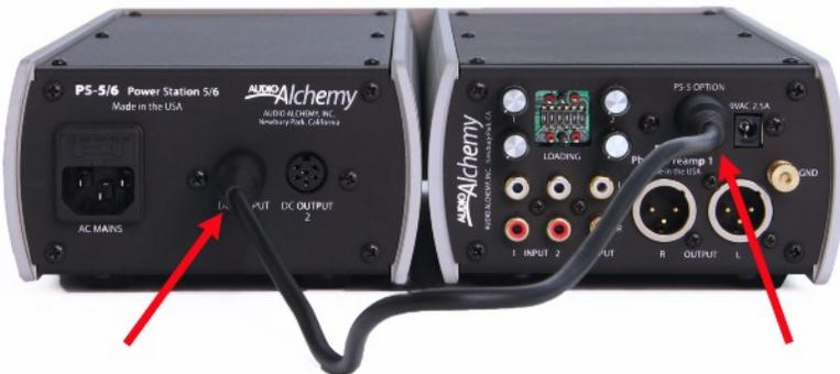
If you are using the optional PS-5 Power Station power supply, plug the cable that comes with the power supply into one of the multipin DC outputs on the back of the PS-5, then into the multipin Power Station input near the lower right corner of the PPA-1. Do not plug the PS-5 into the AC wall socket until you have finished making all audio connections. Be sure to disconnect the stock AC power supply before you connect the PS-5 Power Station.
