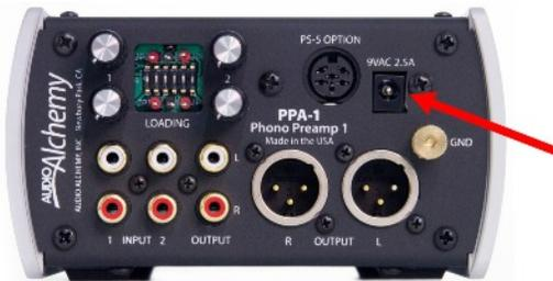
To connect the stock AC power supply that comes with the PPA-1, connect the power supply's cable to the coaxial AC power input on the upper right corner of the back of the PPA-1. Do not plug the power supply into the AC wall socket until you have finished all audio connections. Do not connect the stock power supply if you are using the PS-5 Power Station.
